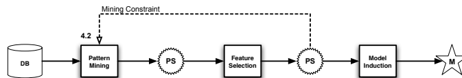
Fig. 3. The model-independent iterative approach: the feedback derived by evaluating the pattern set directly influences the mining of individual patterns.
